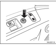
The driver's power window controls also include a lockout button.
